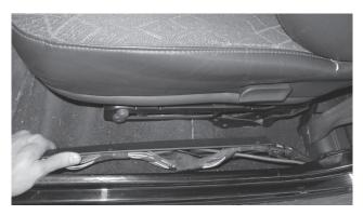
Step 6 - Use a Phillips screw driver to remove the three clips holding the factory wire harness under the door threshold on the driver side.
