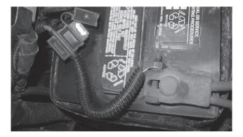
Step 15 - Ground amplifier to chassis of vehicle; connect the terminal provided to the 10ga black wire from furnished wiring harness. A good ground is as important as the power connection. The ground should be as short as possible and the contact point should be free of paint and debris.
