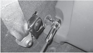
Step 25 - Flip the rear seat back and lock into place against your new enclosure.
