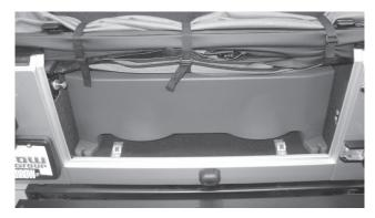
Step 3 - Place enclosure on the floor behind the rear seats with woofers firing down as shown below.
