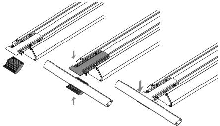
Remove the bolts from the MUDSYSPFCLAMP so the top bracket and MUDSYSPFCLAMP can be properly positioned on the flat portion of the ProFit cage. Once the MUDSYSPFCLAMP are in the proper location for mounting, the bolts should be retightened to a torque specification of 65-70 inch/lbs.
