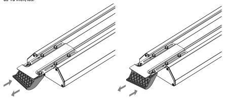
Each MUDSYSPFCLAMP has two (2) total bolts. These bolts can be loosened to adjust the clamp angle allowing it to mount to a variety of roll cages including those that are angled.
